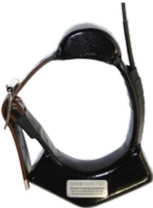
There are currently two data loggers in our range. the RX3-S is the smallest data logger in our range, designed for mammals greater than 2.2Kg, followed by the RX3-SM which is suitable for mammals greater than 5.7Kg. We offer a wide range of optional features to customise collars for specific applications, such as automated timed release.
